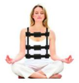
The sound vest is a device that is generally used for pain management. The vest is made up of 9 full range subwoofers that are incased in a wearable vest. All speakers are equally distributed in the front and back side of the body (torso) and is used to send sound frequencies directly into the body.
